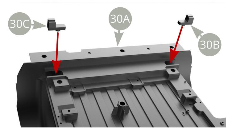
Fit **30C Right** and **30B Left trailing arm return stroke buffers** to the bottom of **30A Chassis rear section** and fix them with two **GM screws** ( top and bottom illustrations ) .
