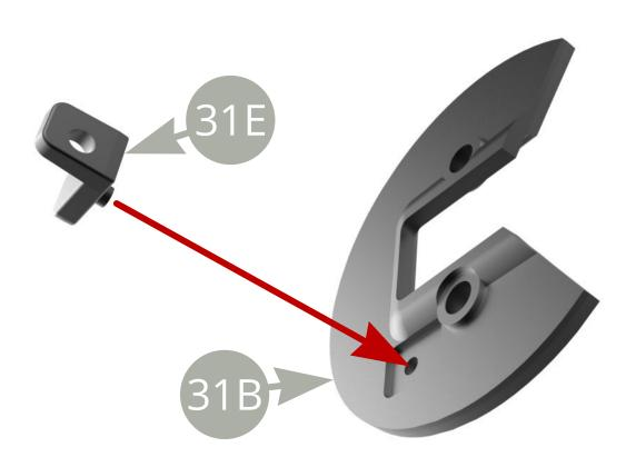
Fit 31E Brake hydraulic hose holder to 31B Brake dust shield.
