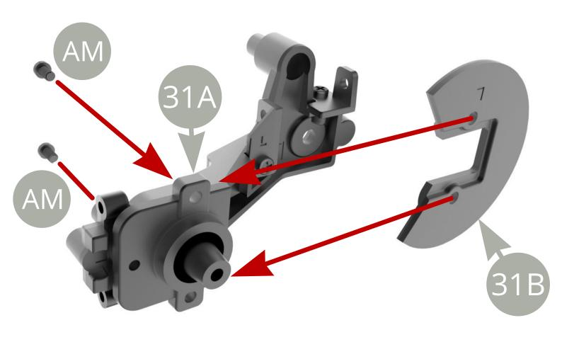
Slide **31B Brake dust shield** to **31A Rear axle left trailing arm**, aligning and fixing with two **AM screws**.
