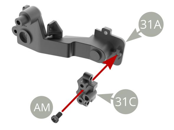
Fit **31C Caliper mounting bracket** to **31A Rear axle left trailing arm** and fix with **AM screw** .
