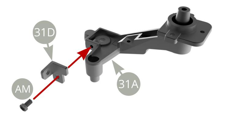
Fit **31D** Handbrake cable holder to **31A** Rear axle left trailing arm and fix with **AM** screw .
