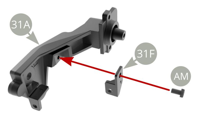
Fit **31F Brake hydraulic hose holder** to **31A Rear axle left trailing arm** and fix with **AM screw** .
