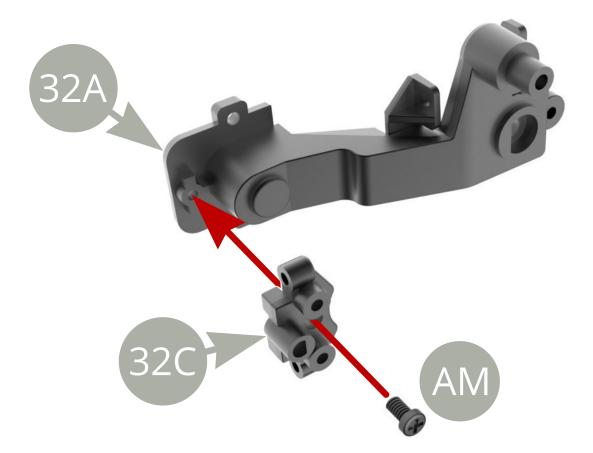
Fit **32C Caliper mounting bracket** to **32A Rear axle left trailing arm** and fix with **AM screw** .
