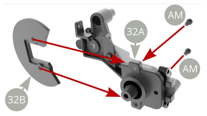
Slide **32B Brake dust shield** to **32A Rear axle left trailing arm**, aligning and fixing with two **AM screws**.
