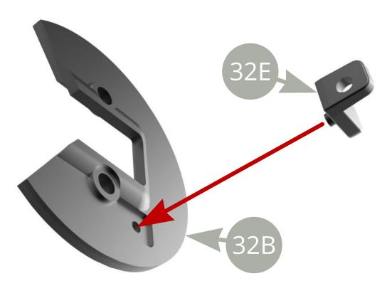
Fit **32E Brake hydraulic hose holder** to **32B Brake dust shield**.
