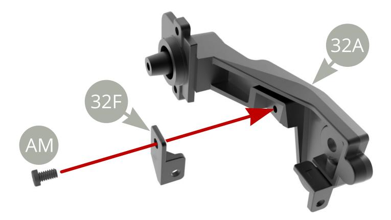
Fit **32F Brake hydraulic hose holder** to **32A Rear axle left trailing arm** and fix with **AM screw** .
