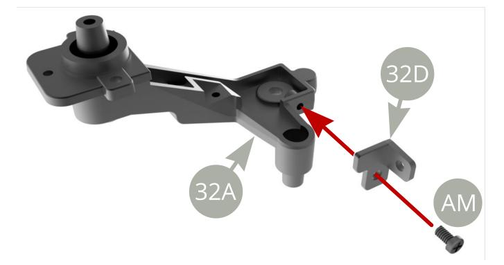
Fit **32D Handbrake cable holder** to **32A Rear axle left trailing arm** and fix with **AM screw** .
